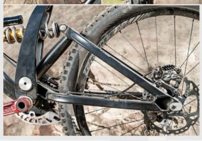
in damping force held the shock up in its travel under larger impacts, causing less buck from the chassis. Without that adjustment, the shock would use its travel quickly, putting undue strain on the wheels and chassis, which would then rebound harshly when snapping back into place. Tuning some progression into the shock helped alleviate those impacts.
